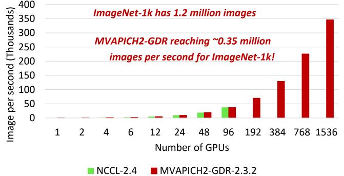
*Platform: The Summit Supercomputer (#1 on Top500.org) – 6 NVIDIA Volta GPUs per node connected with NVLink, CUDA 9.2*
