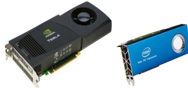
Accelerators / Coprocessors high compute density, high performance/watt
